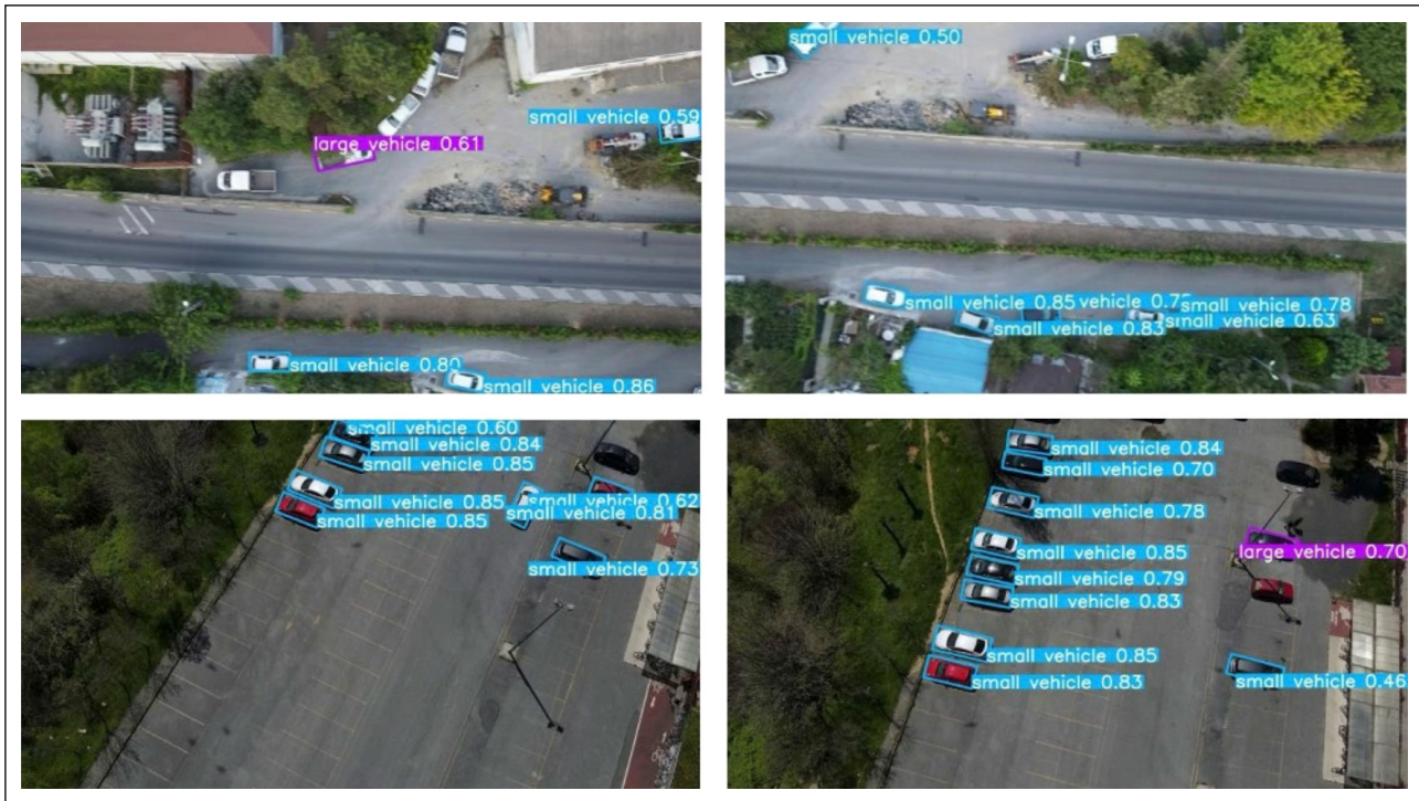
Figure 4. Example images showing passenger cars being detected and enclosed in directional bounding boxes using the YOLO-OBB model. The figure illustrates how the algorithm not only identifies the vehicles but also captures their orientation by aligning the bounding boxes with the direction of the vehicles. This capability significantly improves the robustness of detection compared to traditional axis-aligned bounding boxes, especially in cases where the vehicles are rotated at various angles relative to the drone's field of view. The use of oriented bounding boxes ensures more precise width measurements, which is critical for accurate flight height estimation.
